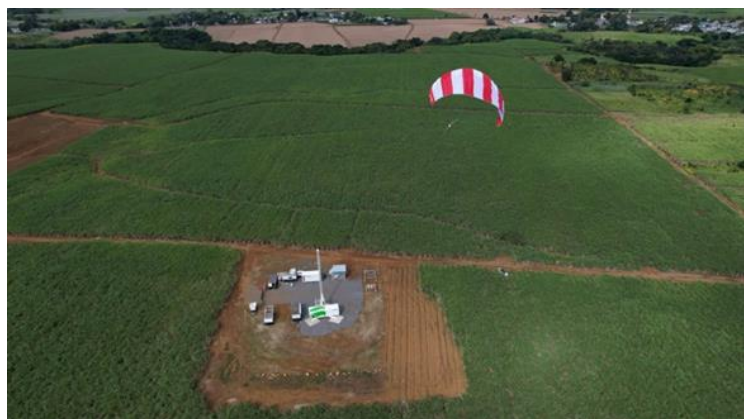
SkySails operating over bagasse fields in Mauritius
